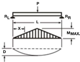
Réaction:  $R_L = R_R = \frac{P}{2}$
