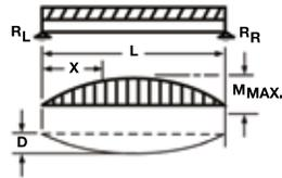
Réaction:  $R_L = R_R = \frac{wL}{2} = \frac{W}{2}$
