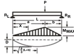
Réaction:  $R_L = \frac{Pb}{L}, R_R = \frac{Pa}{L}$
