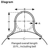
Slots are ½ in. from side to side, and allow for expansion and contraction. Slot dimensions: for sizes 2 in. through 6 in. are ¾ in. wide, ¾ in. long. Slot dimensions: for 1 in. and 1½ in. are ¾ in. wide, ¾ in. long. Slot spacing: 18 in. from center, beginning 6 in. from end.
