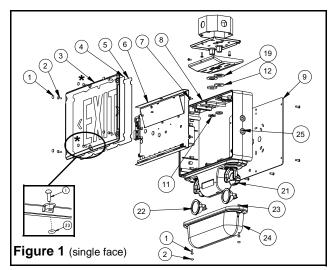
\*Note: Install o-rings (2x) on the screws between the lens and the frame.
