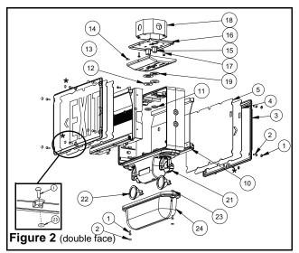
\*Note: Install o-rings (4x) on the screws between the lens and the frame.
