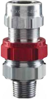
Star Teck Extreme fittings are designed to accommodate a broad range of cables and each hub range overlaps the adjacent hub range, thereby minimizing the possibility of mismatched cables and fittings in the field. They are available in hub sizes from ½ to 4 inches, and will handle outer jacket diameters from 0.525 to 3.870 inches.
