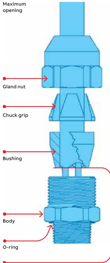
\*When cord will not fit through body, strip cord jacket and trim fillers if required. Insert cable ensuring the outer jacket reaches the end of the bushing as shown. Tighten gland nut onto body
